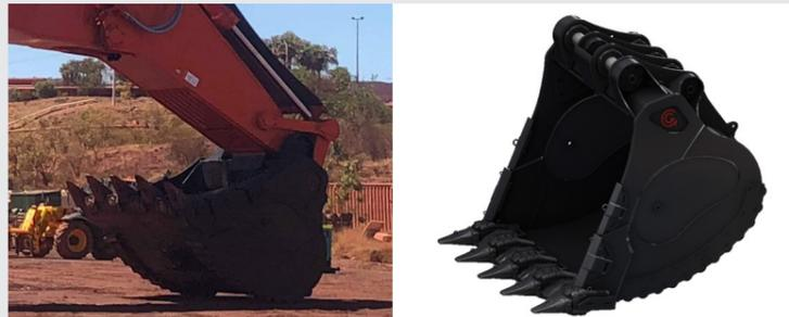
XMOR Backhoe Buckets are proven in operation. The result of years of materials and bucket design knowledge, plus extended field development has resulted in an exceptional combination of wear resistance and strength. Wear parts are minimised, and on-site maintenance reduced with the bucket structure designed to combat wear. XMOR buckets currently available for Backhoes and Wheel Loaders.
